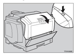
Turn the dial downward, then remove the misfed paper in the printer.
